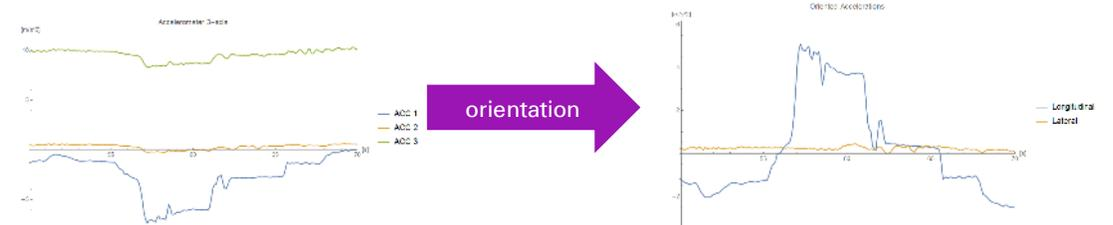
Accelerometer axes are orientated on the vehicle frame in order to have longitudinal, lateral and vertical acceleration of the vehicle.
